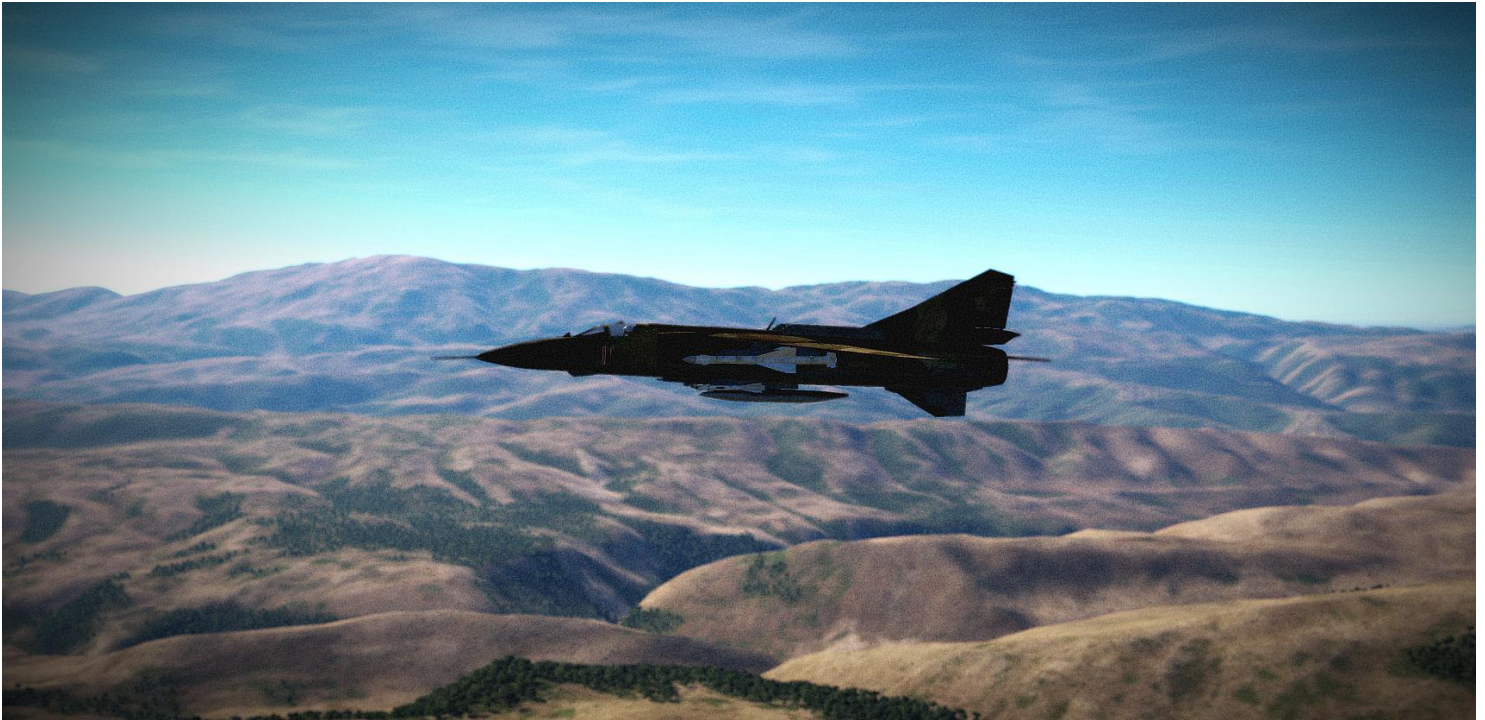
Mig-23 MLD over the Syrian/Lebanese border. Note the R-24 BVR capable missile.
