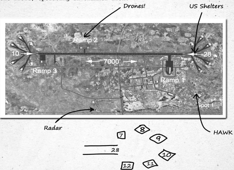
H4 contains 12 hardened shelters, 6 at the east end of the base, 6 at the west. The shelters are connected directly to the runway via short taxiways 45 feet in width. The 79th FS has been assigned the 6 shelters at the east end of the base (Spots 7-12). The base also contains 3 small ramps (Ramp 1, Ramp 2, Ramp 3). H4 houses part of Jordan's air defense network and is equipped with an AN/FPS-117 EW radar and a HAWK battery.
